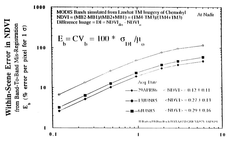
Horizontal Displacement of TM Band 4 relative to TM Band 3
