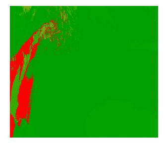
RGB image (no aerosol correction) showing a dust storm (yellow-white) over the Mediterranean sea False RGB image (2.1mic Blue, 1.6mic Green, 3.75mic Red), the low clouds appear whiter than the dust in this false RGB Experimental dust storm mask, the area detected as strong dust concentration are colored in redorange.
