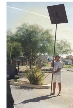
Parasol shaded SWIR measurements (to measure diffuse component)
