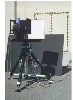
SWIR radiometer viewing sunlit spectralon (both direct and diffuse illumination)
