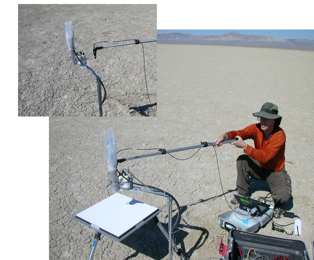
Simultaneous Measurement of Panel with LED Radiometer and ASD - Inset Shows Similar Ground Measurements
