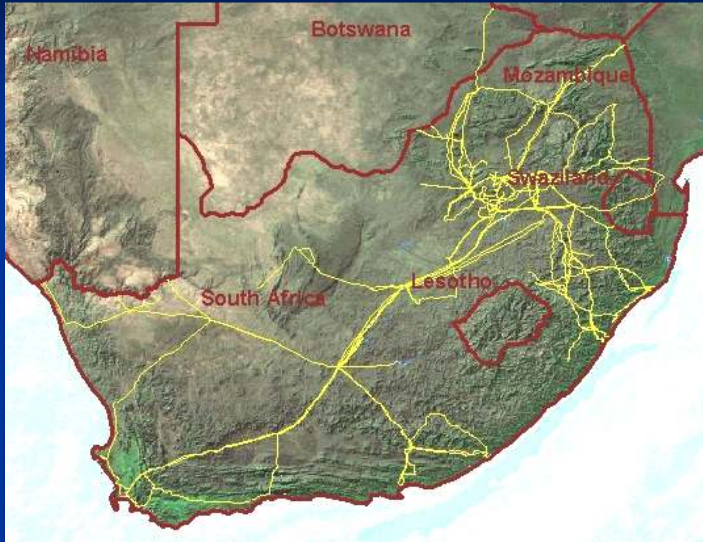
ESKOM transmission network in South Africa
