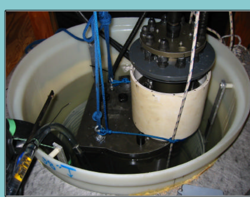
MOS in temperature controlled bath
