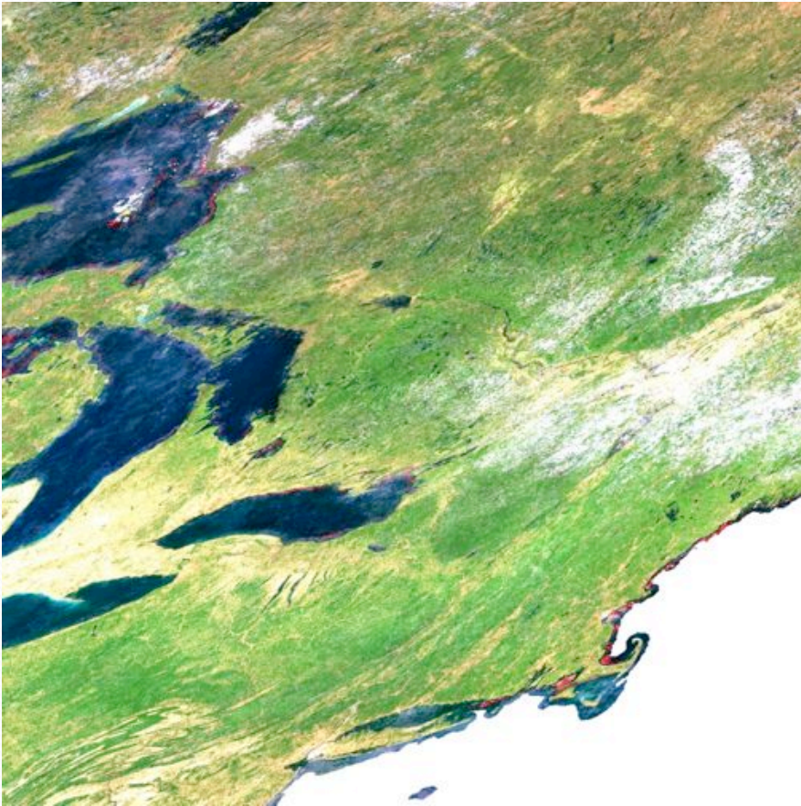
MODIS NBAR product (DOY 145) 2007, original version with white fill values where no retrievals were possible.
