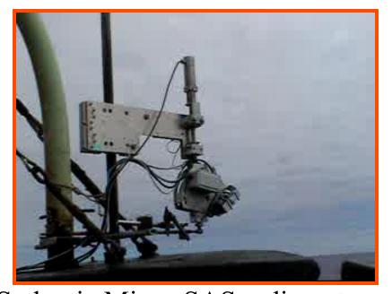
Satlantic Micro-SAS radiometers collect along-track data for Lt, Lsky, and Ed. We designed a mount which compensated real-time for changes in sun's azimuth relative to ship heading.
