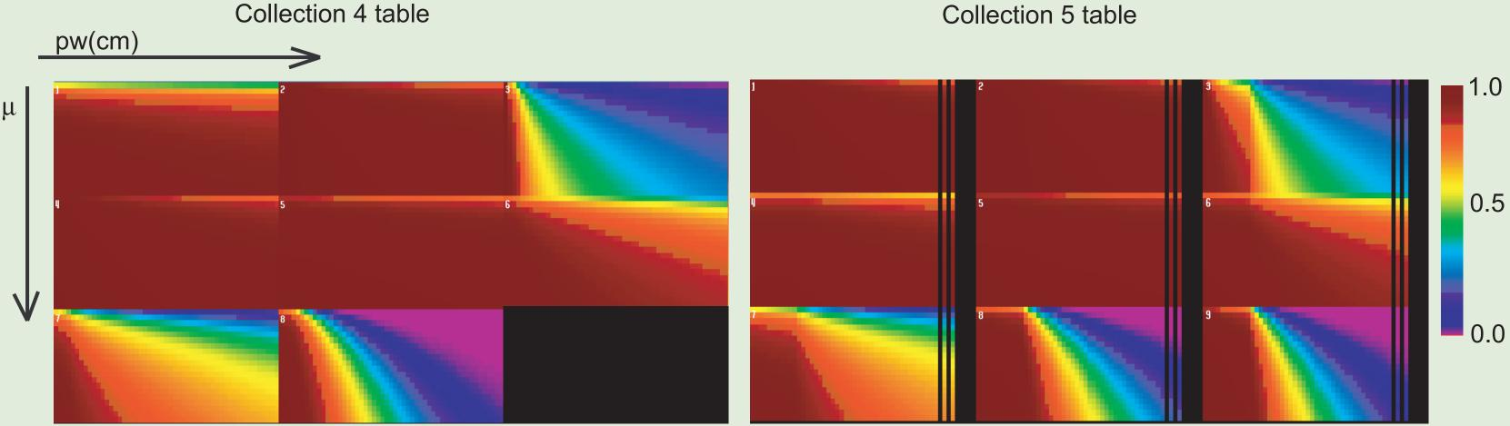
These images illustrate the differences between the new and the old transmittance tables. 11µm band had been added and random MODTRAN ozone profiles had been removed from 0.65µm band transmittance. The new table had been re-gridded to give finer resolution between 0.0 and 0.2 cm of precipitable water. The new table was generated using the ECMWF 13,000 profile database.
