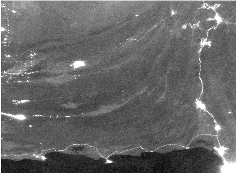
2014 DNB Composite over Southern Pakistan – some road features have lower average radiance values than no-light areas with high albedo
